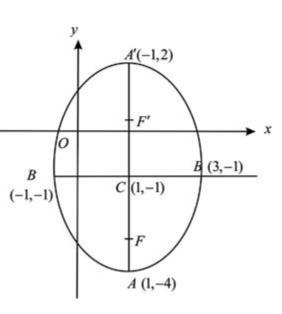
**Example 4.** An arch in the form of half an ellipse is 40 m wide and 15 m high at the centre. Find the height of the arch at a distance of 10 m from its centre.
