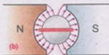
Fig. 14.19 (a) Moving coil (b) Concave pole piece and soft iron cylinder to produce radial and stronger
