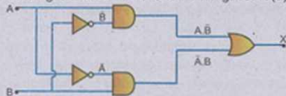
Fig. 18.40 (a) Making an XOR gate
