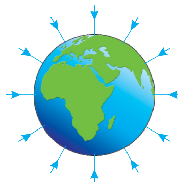
Figure 5.3: Gravitational field around the Earth is towards its centre.
