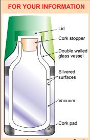
In a thermos flask, most of the heat is prevented to enter or leave the flask. This is done by suitable measures to reduce the transfer of heat due to conduction, convection and radiation. Thus, anything kept in it, maintains its temperature for a long time.
