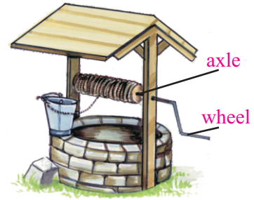
Fig.9.6: The crank on the well is a kind of wheel and axle. It reduces the force needed to raise the bucket.
