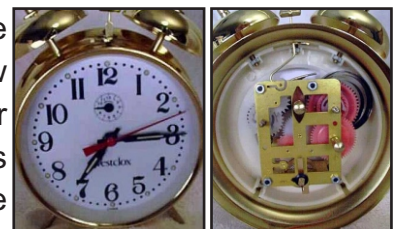
Fig.9.17: Gear system in a wind-up clock
