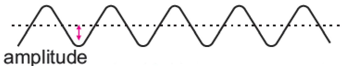
Fig.10.11: Waves of a soft sound have small amplitudes.
