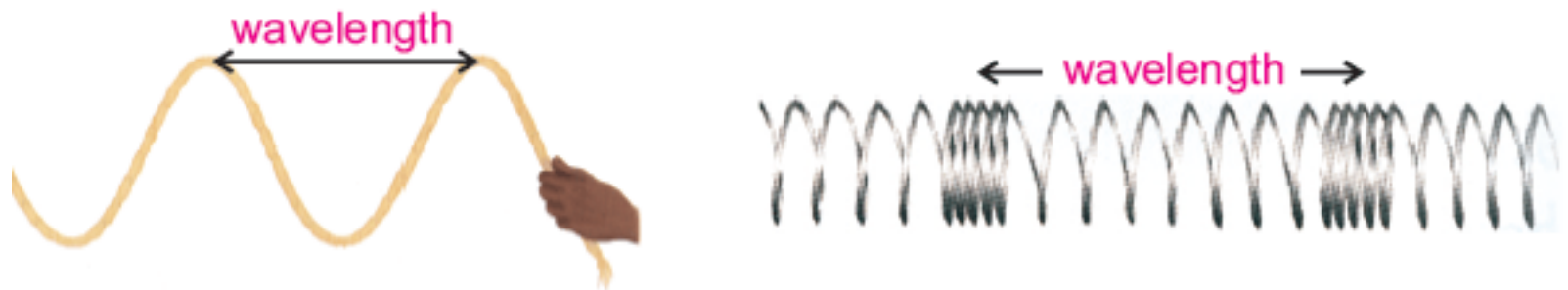
Fig. 10.5: Distance between two adjacent crests or compressions is the wavelength.
