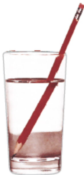
Fig. 9.1: The pencil in the glass of water looks as it has been broken at the water line. It is because of refraction of light.
